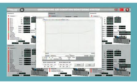
The operating modes, operating data, operating status, operating time settings, alarms, scenario, parameter, and system settings, air handling unit details, energy analyzer, and energy consumption details are displayed via various screens.
