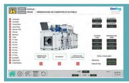
GAHU devices have a preinstalled, preconfigured and fully integrated control system with a wall-mounted control panel.
